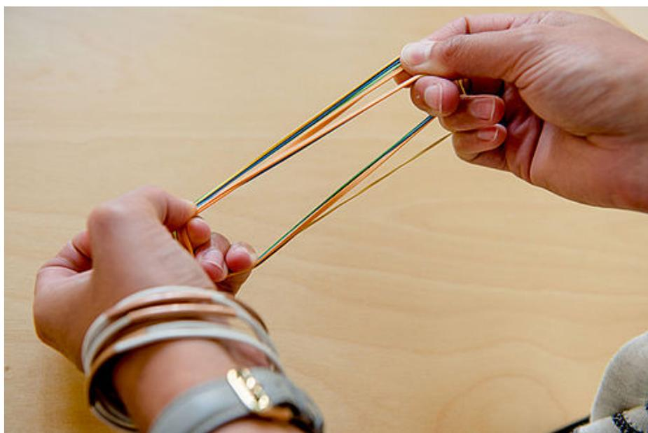
*If one bends rubber bands again and again, the sulphur bridges in the material break. The rubber becomes brittle. © RUB, Marquard*
